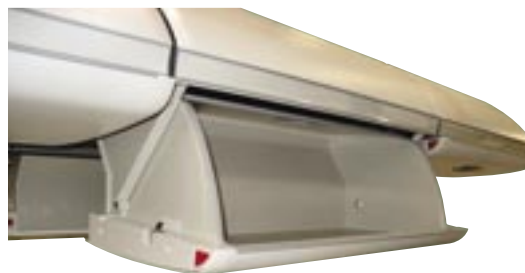
Stow bin made with Cetex 3 system
