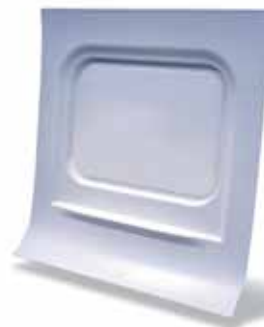
Train window mask from Azdel® Rail-Lite® composite used on the Long Island Railroad, New York. Azdel Rail-Lite composite, a breakthrough technology from Azdel, Inc., and SABIC Innovative Plastics, is a new low-pressure, thermoformable, lightweight composite sheet that exhibits excellent flame, smoke, toxicity, and heat-release performance in large semi-structural train panels.
