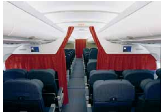
Adder cabin divider SABIC Innovative Plastics provided parts made from Ultem® 1668 sheet to Airbus aircraft for the development of Adder cabin dividers.
