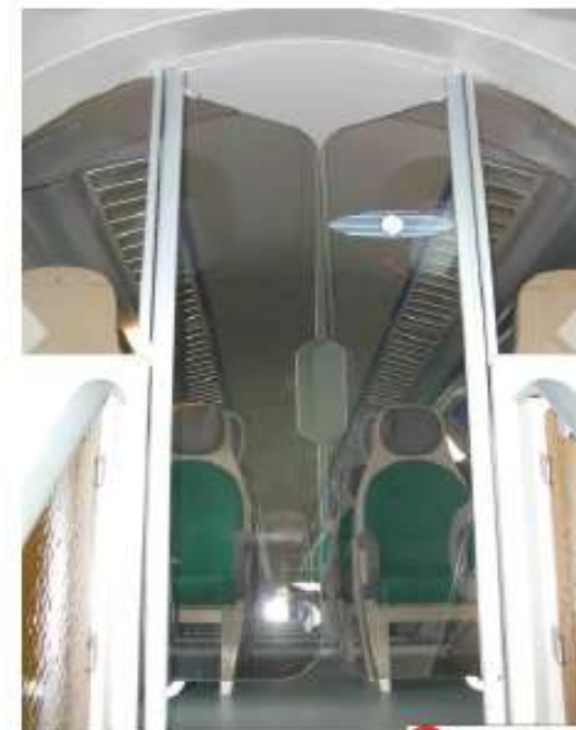
Italian railways compartment separators Using LEXAN MARGARD sheet.
