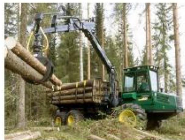
Old type JD cabin for forwarder Using flat Lexan MR5E 12mm
